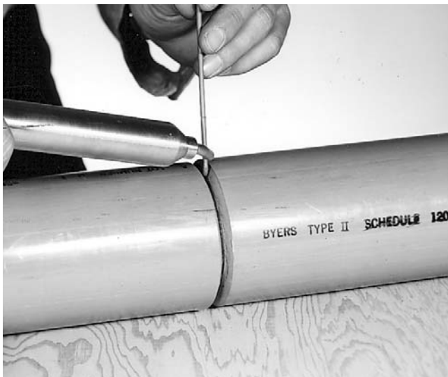
Butt Welding PVC Pipe
