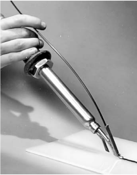
Speed Welding Polyethylene Sheet
